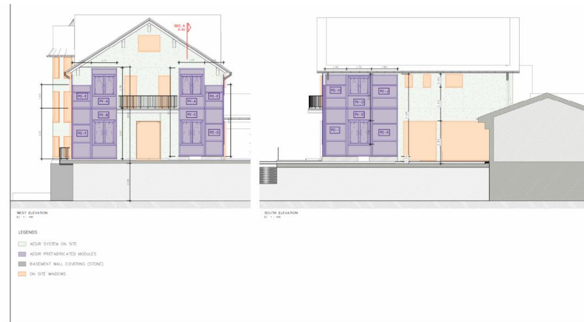
FA-02 | AEGIR Modules - Elevations II
